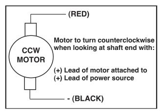
Power supply wiring must conform to all required safety codes and be installed by a qualified person. Check that supply voltage agrees with that listed on product nameplate. Minimum supply wire gage: 14 AWG.
